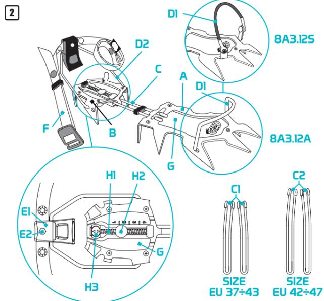
**EN:** (A) carbon steel Front frame, (B) carbon steel Back frame, (C) stainless steel connecting shaft: (C1) sizes EU 37-43 and (C2) sizes EU 42-47, (D) stainless steel Binding shaft (D1) front (for the semi-automatic version it is in PVC coated steel) and (D2) back, (E1) Nylon Heel pad and stainless steel screw (E2), (F) Nylon safety loop with Aluminium buck, (G) Polyamide Antibott, (H) Adjusting system: (H1) Stainless steel screw, (H2) Aluminium Regulating Nut, (H3) Rubber Blocking Nut.
